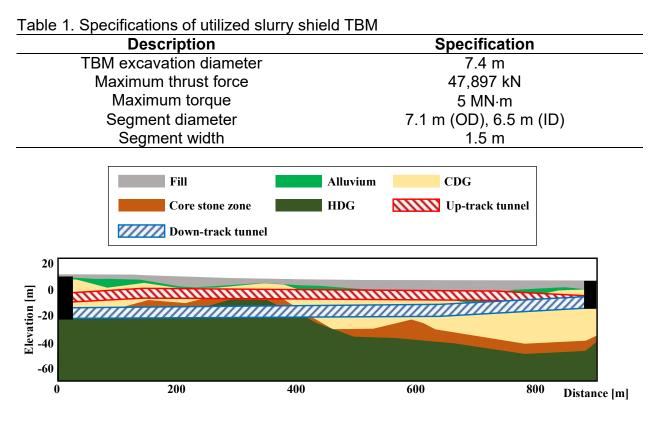
Fig. 1 Longitudinal geological profile of the site
